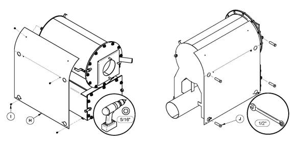
**Step 6.** Remove the vision tube cap.
