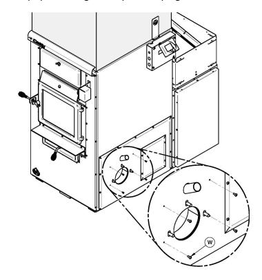
Step 14. Install the burner (AA). Secure it with washers (Y) (3X) and nuts (Z) (3X) (Beckett unit).
