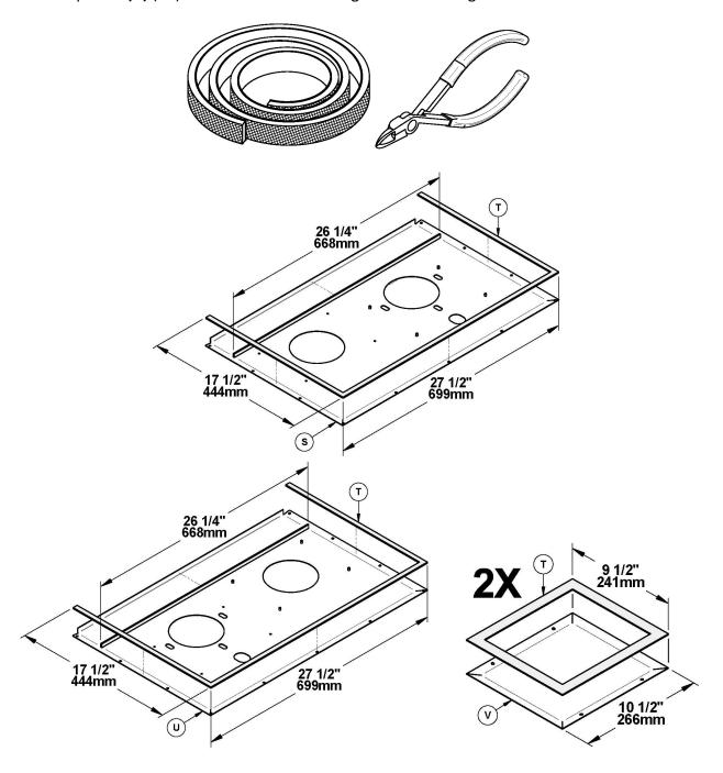
Step 10. Install the air jacket panels (V) (2X) on the left (S) and right (U) panel with the screws (W) (8X).
