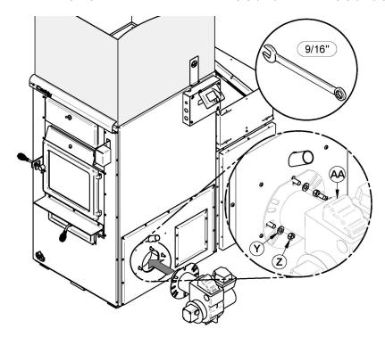
Install the burner (BB). Secure it with washers (Y) (3X) and nuts (Z) (3X) (Riello unit).
