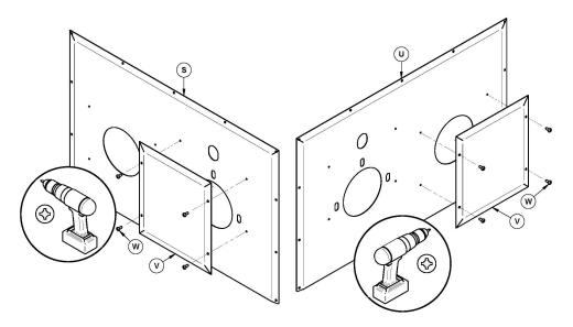
**Step 11.** Install the left panel **(S)** on the furnace. Secure it with the screws **(C)** (11X) removed from **Step 1**. Plug the panel holes with the screws provided with the oil unit.
