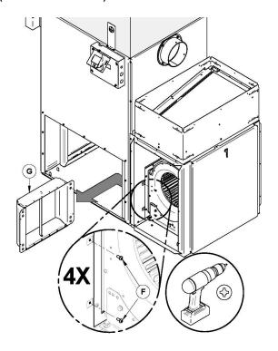
**Step 4.** Replace the right and left blower box panels **(D)** with screws **(E)** (18X). (Note: If the blower box wasn't already installed on the furnace, the missing screws (12X) can be found in the blower box user's manual kit).
