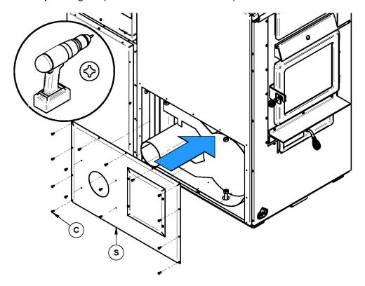
**Step 12.** Install the gasket **(X)** on the oil unit combustion chamber cover. Then install the right panel **(U)** with the screws **(C)** (11X) removed from **Step 1**.
