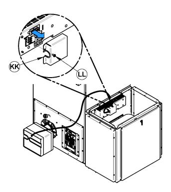
To facilitate connections, the use of a junction box is recommended. It can be installed on the back of the furnace. Use the following diagram for reference. Refer to the wiring diagram for complete connections.
