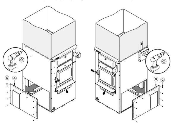
**Step 2.** Remove the right and left panels of the blower box **(D)** by removing the screws that hold them in place **(E)** (6X if the blower box wasn't already installed on the furnace, 18X if the blower box was already installed on the furnace). Keep the screws.
