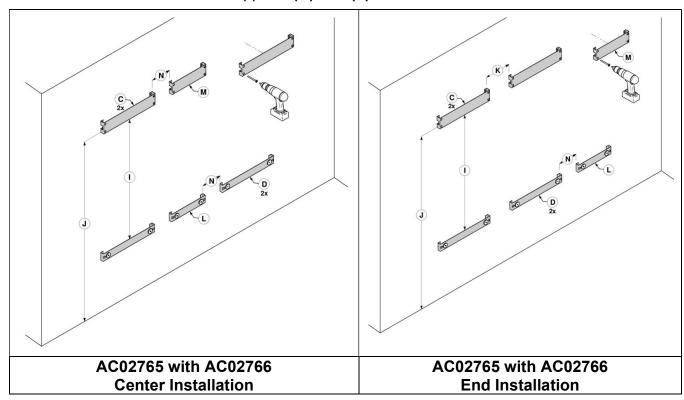
4. Position and fix the bottom supports (D) and (L) with anchors and screws.
